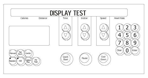
Upon entry to this test, all lights will be turned ON. This test will allow the user to test the display console.
